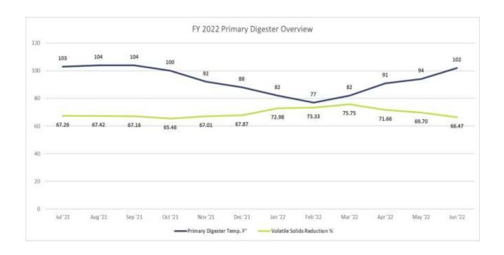
During FY 2022, the digester process produced a total of **9,770,800** Cubic Feet of Methane Gas. Of this amount, **6,917,400** Cubic Feet used by the boiler system to maintain digester temperature, the remaining **2,853,400** Cubic Feet of gas was burnt off through the candle ignition system.
