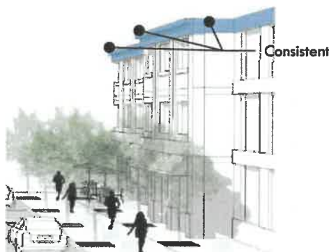
Figure. Roof Parapet and Cornice Lines
